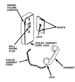
Figure 4. Wall Telephone Installation
